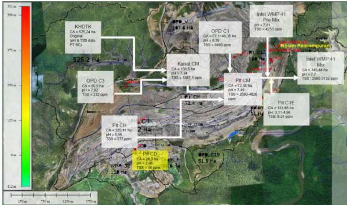
Gambar 1. Sistem Dewatering Tambang Pit C1 Blok 8 BMO 2 PT Berau Coal 2022.
